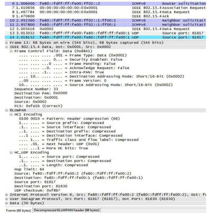
Figure 7. Example of using Wireshark to analyze captured UDP packet sent over the IEEE 802.15.4 standard
