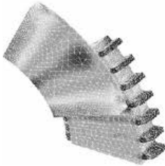
Fig. 4. Magnetic field distribution in the machine.
