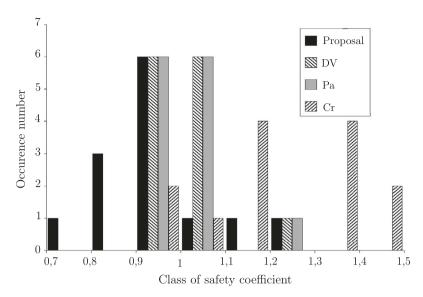
Fig. 9. Comparison of the safety coefficients for the constant amplitude fatigue tests under the combined tension and torsion with internal pressure on smooth specimens of St35 steel (DV = DangVan, Pa = Papadopoulos, Cr = Crossland) [29].
