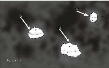
**Fig. 5.** Schematic 2D illustration of the damage parameter  $W_{g_{eq}_{dom}}$ . Critical points and illustration of the volumes influencing fatigue crack initiation.
