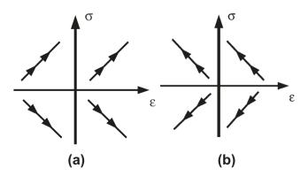
**Fig. 2.** Elastic strain stress paths that corresponds to a positive values of the strain work density increment.
