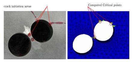
Fig. 16. Comparison between the experimental fatigue crack initiation sites and the critical points computed by the proposed method.
