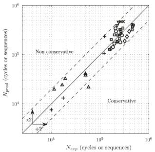
**Fig. 10.** Experimental and simulated fatigue lifes (for in service loadings fatigue life is expressed in number of load sequences) for different loading cases on EN-GJS800-2 smooth specimens.
