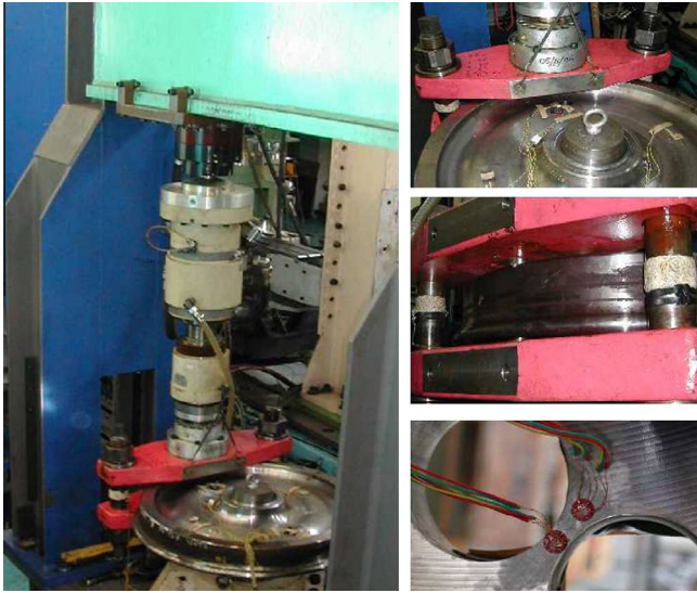
Fig. 14. Drilled wheel on SNCF-AEF fatigue test bench.
