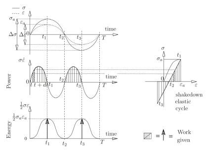
**Fig. 1.** Illustration of work and elastic strain power given to an elementary volume element, during a loading period *T* (with the assumption of elastic shakedown) under fully reversed tension.
