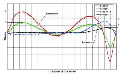
Fig. 13. Variable amplitude combined tension and torsion load history and illustration of the magnification factor k.
