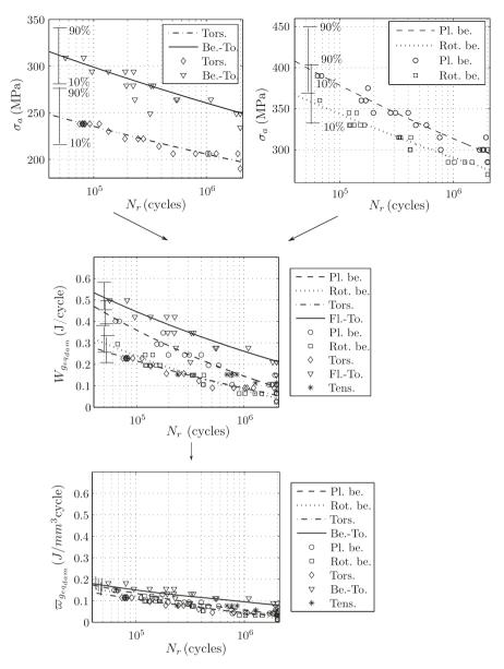
**Fig. 6.**  $W_{g_{eq,dam}}$  and  $\varpi_{g_{eq,dam}}$  evolutions according to the median fatigue life for various loadings for ER7 steel.
