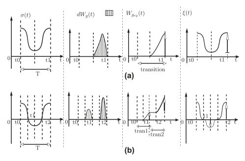
Fig. 3. Stress, incremental and cumulated damage parameter and energy function evolution under uniaxial tensile loading for positive an negative loading ratio.
