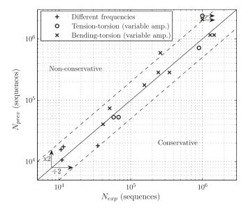
**Fig. 12.** Comparison of experimental and simulated fatigue lifes with fatigue life calculation method on different fatigue tests on ER7 steel smooth specimens.
