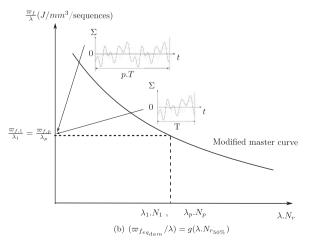
Fig. 4. (a) Usual and (b) Modified master curve representation.
