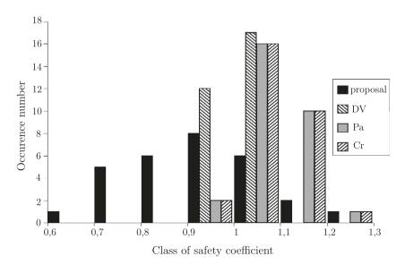
Fig. 8. Safety coefficients distributions for the constant amplitude fatigue tests under combined rotative bending and torsion on smooth SAE1045 specimens (DV = DangVan, Pa = Papadopoulos, Cr = Crossland) [28].
