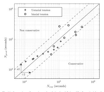
**Fig. 11.** Comparison of experimental and simulated fatigue lifes for uniaxial and biaxial variable amplitude fatigue tests on 10HNAP steel.
