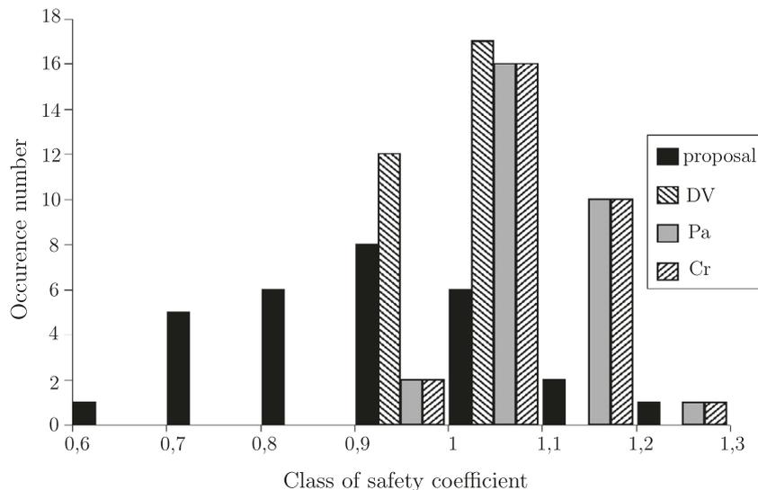
**Fig. 8.** Safety coefficients distributions for the constant amplitude fatigue tests under combined rotative bending and torsion on smooth SAE1045 specimens (DV = DangVan, Pa = Papadopoulos, Cr = Crossland) [28].
