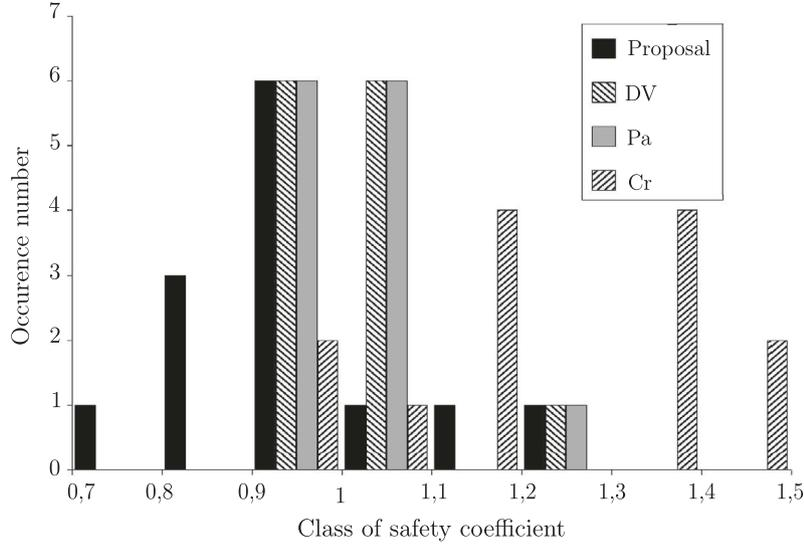
**Fig. 9.** Comparison of the safety coefficients for the constant amplitude fatigue tests under the combined tension and torsion with internal pressure on smooth specimens of St35 steel (DV = DangVan, Pa = Papadopoulos, Cr = Crossland) [29].
