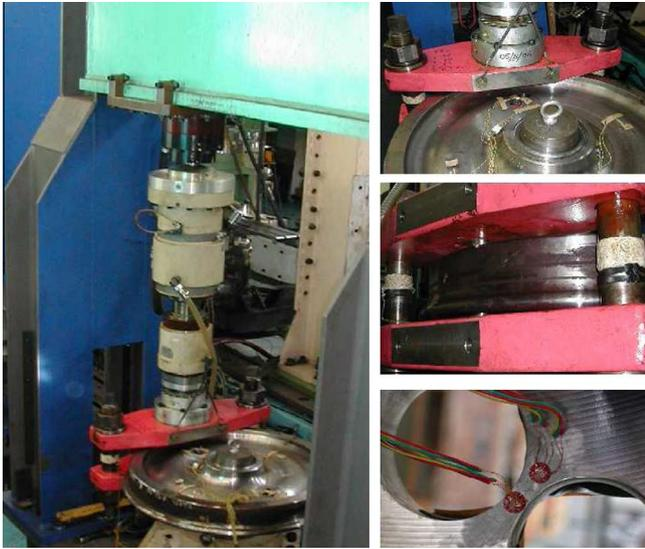
Fig. 14. Drilled wheel on SNCF-AEF fatigue test bench.
