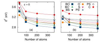
FIG. 3. Uncorrected (a) and corrected (b) Zr SIAs formation energies  $E^{\rm f}$  of the stable configurations versus the number of atoms for  $\varepsilon = 0$  calculations.
