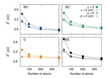
FIG. 2. Formation energies  $E^{\rm f}$  of the four most stable SIAs in Zr versus supercell size. Filled symbols refer to ab initio uncorrected results and open symbols to the results corrected by the elastic model. The periodicity vectors of the supercell have been either kept fixed (square) or relaxed (triangles) in the ab initio calculations.
