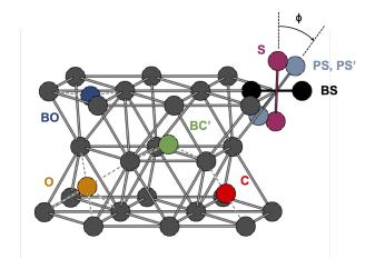
FIG. 1. Structures of the stable SIA configurations in hcp Zr: Octahedral (O), basal octahedral (BO), split dumbell (S), basal split dumbell (BS), crowdion (C) and buckled basal crowdion (BC'). PS and PS' are obtained by a rotation of angle  $\phi = 30^{\circ}$  and  $50^{\circ}$  of S in the prismatic plane.<sup>26</sup>
