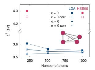
FIG. 6. Vacancy formation energy  $E^{\rm f}$  in silicon calculated with the LDA and HSE06 functionals, either for fixed periodicity vectors ( $\varepsilon = 0$ ) or at zero stress ( $\sigma = 0$ ). Filled symbols refer to the ab initio uncorrected results and open symbols to the results corrected by the elastic model. The vacancy configuration is displayed in the inset: the white sphere corresponds to the empty lattice site and the purple spheres represent its first nearest neighbors.
