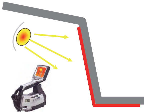
Fig. 19. Schematic representation of the survey area by active infrared thermography.
