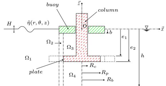
Fig. 1. Definition sketch of the Wave Energy Converter.
