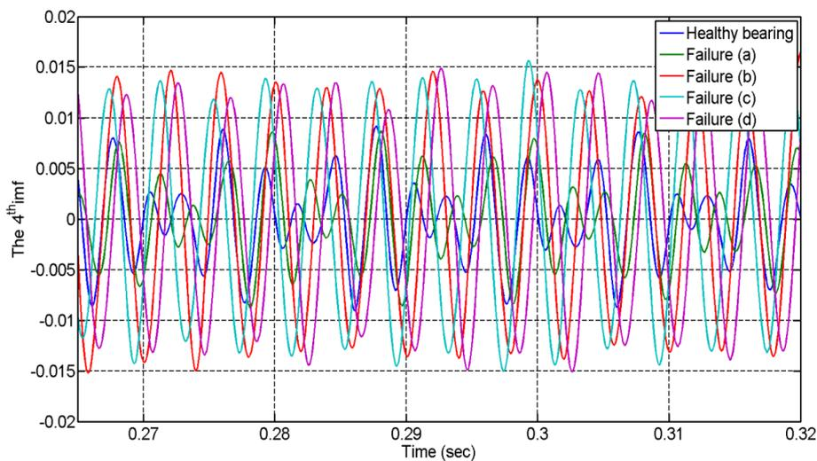
**Fig. 12.** Homopolar current 4<sup>th</sup> IMF for healthy and faulty bearings.
