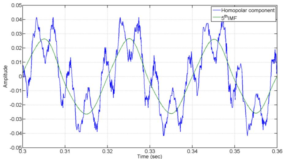
**Fig. 15.** Homopolar current and its 5<sup>th</sup> IMF for faulty bearings.
