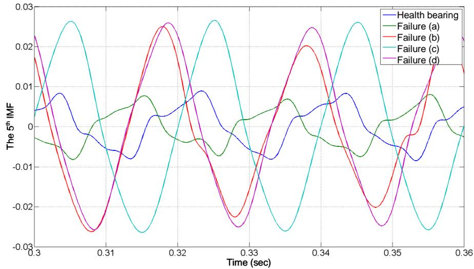
**Fig. 16.** Homopolar current 5<sup>th</sup> IMFs for healthy and faulty bearings.
