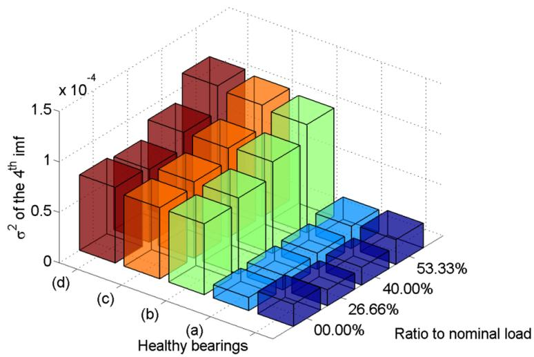
**Fig. 13.** Homopolar current 4<sup>th</sup> IMF variance for healthy and faulty bearings.
