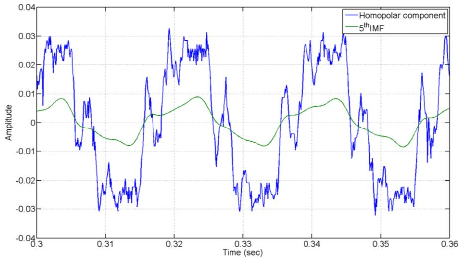
**Fig. 14.** Homopolar current and its 5<sup>th</sup> IMF for healthy bearings.
