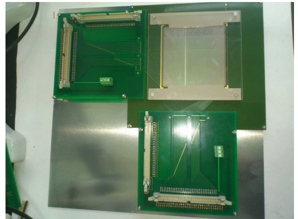
Fig. 6. Large silicon detector with 2 \times 64 strips mounted on a test board.
