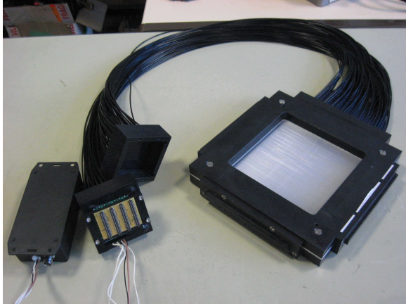
Fig. 11. The beam tagging hodoscope with 2 \times 128 scintillating fibers
