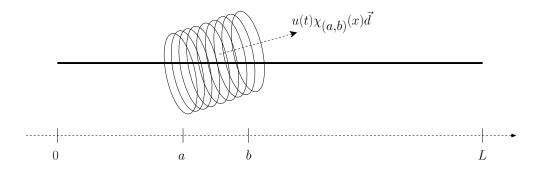
Figure 2: The solenoid used as controller
