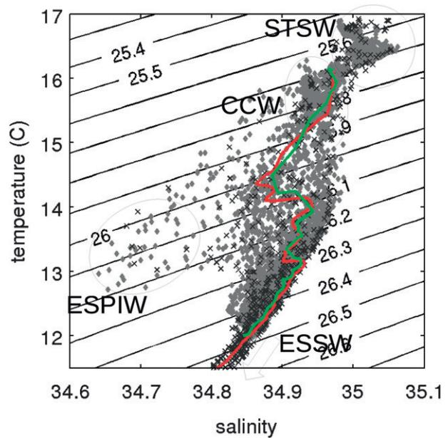
FIG. 2. The  $\Theta$ – $S$  diagram from glider section 2 data (diamonds) and from R/V *Olaya* CTD data along the glider track (crosses). Green and red lines indicate the closest profiles (3.8 km and 1h 30 min) from the glider and the ship, respectively.
