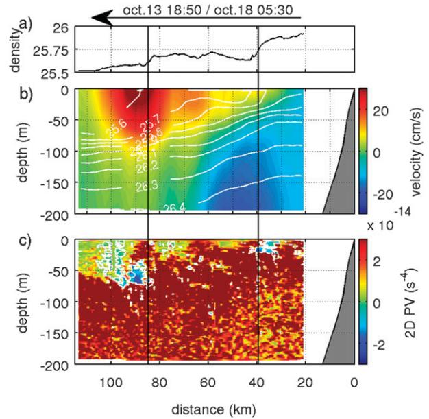
FIG. 10. (a) Cross-shore surface density profile, (b) absolute geostrophic velocity perpendicular to glider section #3 (color coded,  $\text{cm s}^{-1}$ ). Smoothed density contours are indicated by white lines. (c) 2D potential vorticity  $q$  (color coded,  $\text{s}^{-4}$ ) from glider section #3 with white contour corresponding to  $q = 0 \text{ s}^{-4}$ . Vertical black lines mark the position of the most pronounced surface density fronts.
