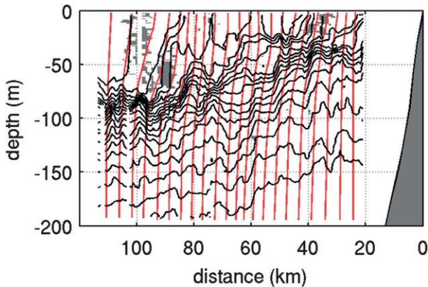
FIG. 11. Absolute momentum surface (red contours,  $\text{m s}^{-1}$ ) and density (black contours,  $\text{kg m}^{-3}$ ) for glider section #3. Contour intervals are  $0.15 \text{ m s}^{-1}$  for absolute momentum and  $5 \times 10^{-2} \text{ kg m}^{-3}$  for density. Zones of negative PV are marked in gray.
