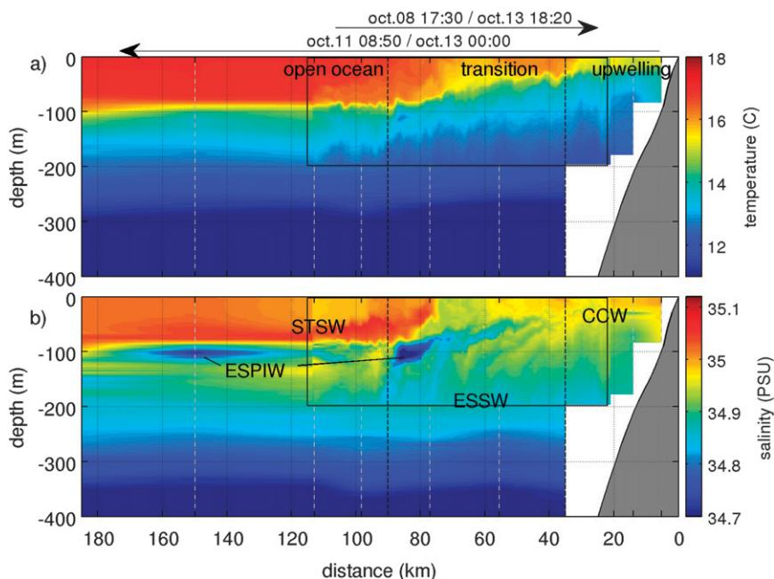
FIG. 5. Vertical sections of (a) potential temperature and (b) salinity carried out from R/V *Olaya* between 11 and 13 Oct along a section contiguous to the glider sections. The glider section #2 (8–13 Oct) is superimposed in the black rectangle. Three regions (offshore, transition, and coastal) are delimited by black dashed lines. Ship CTD casts are indicated with thin gray-dashed lines.
