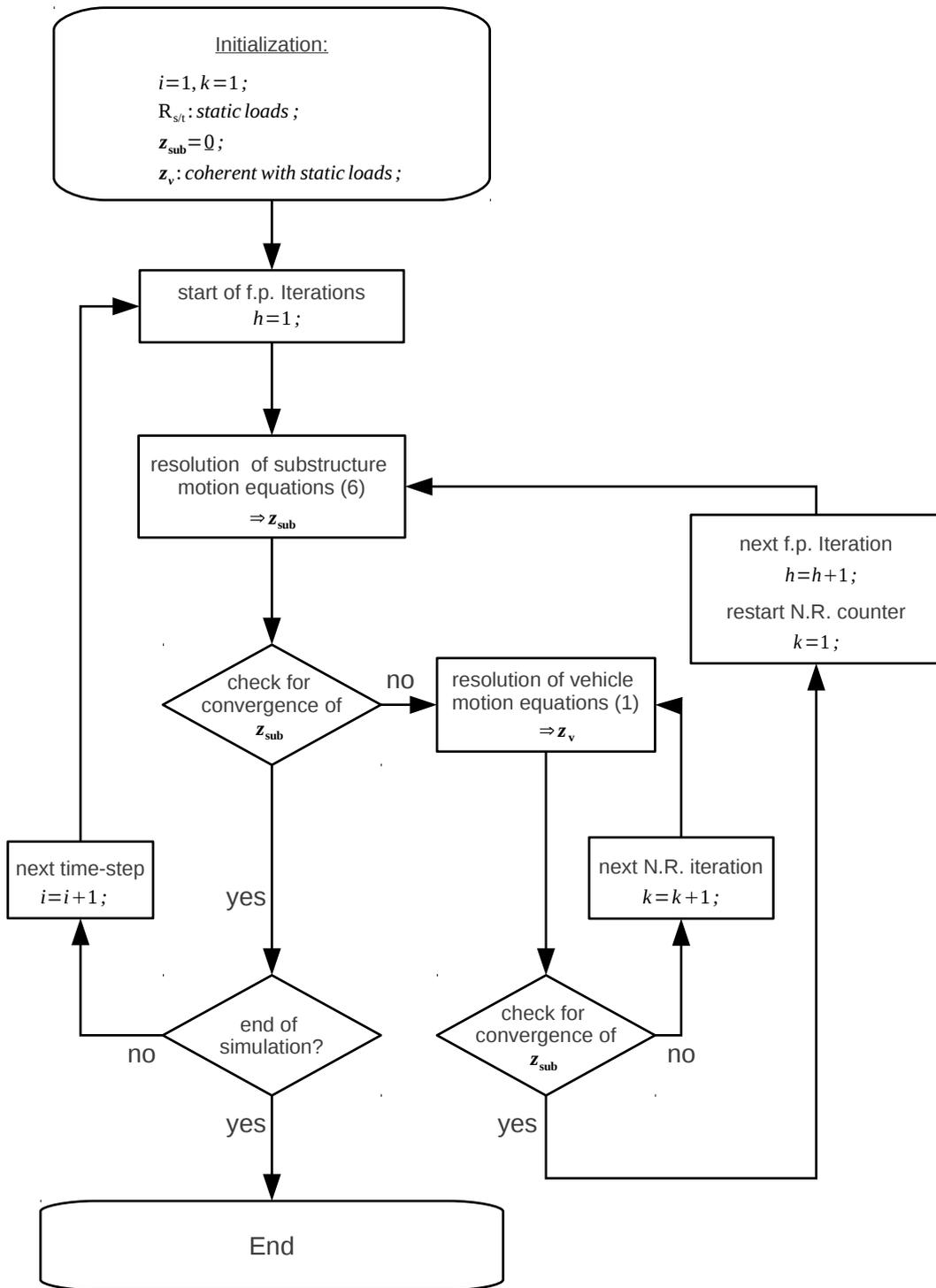
Figure 2: Algorithm of resolution.
