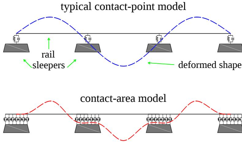
Figure 3: Draft of rail deformed shape in the case of the contact-point model and contact-area model.
