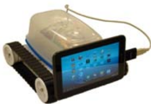
Figure 1. Robot: Rover 5 base + Phidget (inside the box)+ Tablet PC
