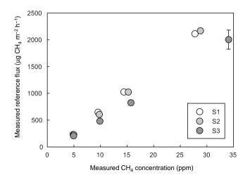
**Fig. 2.** Measured reference fluxes of  $CH_4$  against measured  $CH_4$  concentrations inside the calibration tank at the start of each chamber measurement during the whole measurement campaign. Colors represent concentrations for dry fine sand (S1), dry coarse sand (S2) and fine wet sand (S3). Bars denote standard errors of the mean. Note that the bars of the measured  $CH_4$  concentration are too small to be visible.
