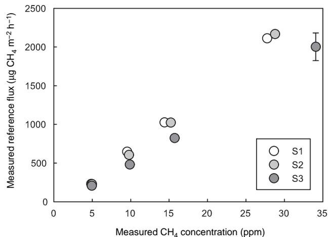
**Fig. 2.** Measured reference fluxes of CH<sub>4</sub> against measured CH<sub>4</sub> concentrations inside the calibration tank at the start of each chamber measurement during the whole measurement campaign. Colors represent concentrations for dry fine sand (S1), dry coarse sand (S2) and fine wet sand (S3). Bars denote standard errors of the mean. Note that the bars of the measured CH<sub>4</sub> concentration are too small to be visible.
