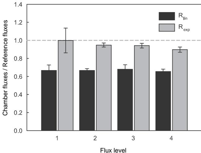
**Fig. 4.** Relation of mean chamber fluxes to mean reference fluxes for four different flux levels. All 15 chambers and 3 sand types are included and values are given for fluxes calculated by the linear ( $R_{lin}$ ) and exponential ( $R_{exp}$ ) flux calculation methods. On the Y-axis the value 1 represents the value where chamber fluxes equal the reference fluxes (no under- or overestimation). Error bars represent standard errors of the means.
