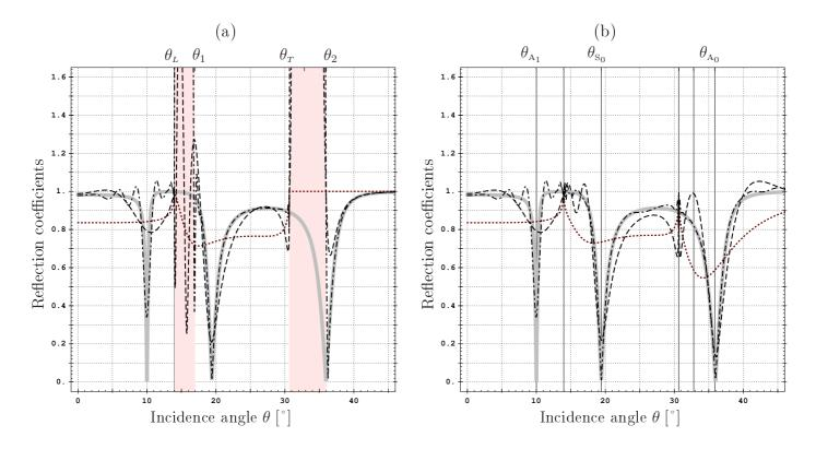
Figure 5: Convergence study for a dimensionless half-thickness  $h = \omega \, h \, / \, c_T = 2 \, (a)$  in the exponential basis and (b) in the orthogonal symmetric basis  $(z_{\alpha} = 0 \ for \ all \ \alpha)$ . The absolute value of the global reflection coefficient |r| (plain) is compared to  $\left| \sum_{n=0}^{n_{\text{max}}} r_{2n} \right|$  for  $n_{\text{max}} = 0$  (first reflection, dotted),  $n_{\text{max}} = 2$  (dashed) and  $n_{\text{max}} = 10$  ( $-\cdot$ ).
