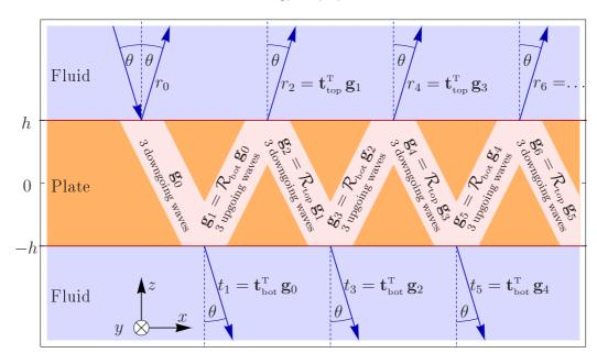
Figure 2: Successive reflections/refractions in an immersed plate.
