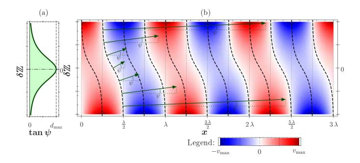
Figure 3: (b) Magnitude of non-zero coordinates of nonstandard progressive waves in isotropic elastic media. The dashed lines correspond to wavefronts. (a) Tangent of the angle  $\psi$  between the normal of the wavefronts and the x-axis:  $\tan \psi = d_{\max}/\cosh(2 \delta \mathbb{Z})$ .
