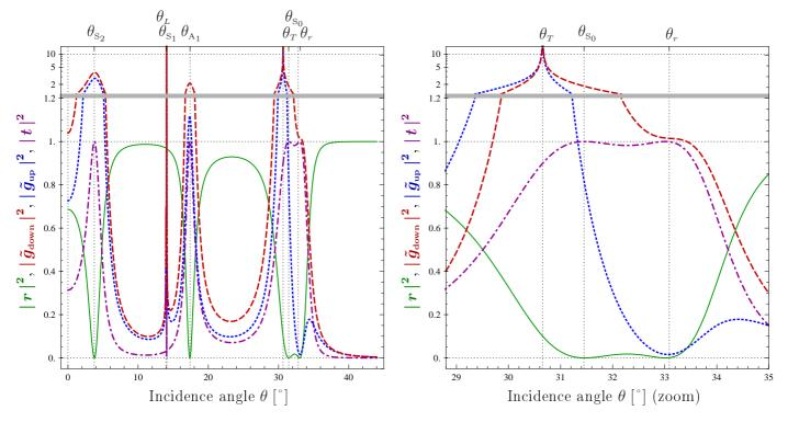
Figure 9: Global coefficients:  $|r|^2$  (reflection, solid),  $|t|^2$  (transmission, dash-dot),  $|\tilde{\mathbf{g}}_{up}|^2$  (upgoing energy, dotted) and  $|\tilde{\mathbf{g}}_{down}|^2$  (downgoing energy, dashed) for the dimensionless half-thickness  $\hbar \approx 3.602$ , in the orthogonal symmetric basis ( $\mathbb{Z}_{SV} = \mathbb{Z}_P = 0$ ).
