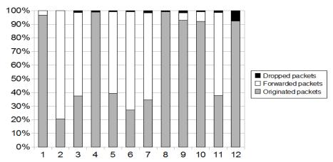
To improve knowledge about propagation inside the vessel, paths followed by packets from source nodes towards the base station have been studied. As previously stated, the sensor nodes are pre-programmed by the Crossbow XMesh routing protocol. Therefore, a sensor node selects the next hop which minimizes the number of transmissions required to send a
