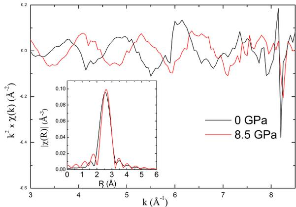
FIG. 3.  $\text{Ce}_{60}\text{Al}_{20}\text{Cu}_{20}$   $k^2$ -weighted EXAFS functions  $k^2 \times \chi(k)$  ( $\text{Å}^{-2}$ ). Inset: the corresponding amplitude of the FT  $|\chi(R)|$ .
