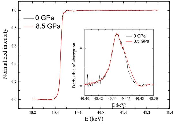
FIG. 2. Ce K-edge x-ray absorption spectrum of  $\text{Ce}_{60}\text{Al}_{20}\text{Cu}_{20}$  bulk metallic glass at ambient conditions (black curve) and 8.5 GPa (red curve). Inset: Corresponding derivative of absorption at 0 GPa (black curve) and at 8.5 GPa (red curve).
