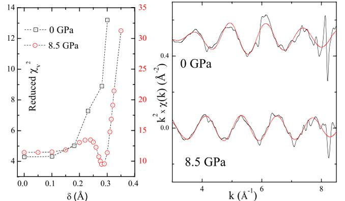
FIG. 4. Left:  $\chi_v^2$  as a function of  $\delta$  parameter (splitting of the Ce-Ce distance in  $\text{Ce}_{60}\text{Al}_{20}\text{Cu}_{20}$  metallic glass). Right: best fit (red) to EXAFS data  $k^2 \times \chi(k)$  ( $\text{Å}^{-2}$ ) (black) at 0 GPa (up) and 8.5 GPa (down).
