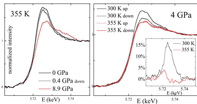
FIG. 6. Left: Ce  $L_3$ -edge XANES of  $Ce_{69}Al_{10}Cu_{20}Co_1$  metallic glass at 355 K. Black: ambient, red: high P, dashed: after decompression. Right: XANES spectra on  $Ce_{69}Al_{10}Cu_{20}Co_1$  at 300 K (black) and at 355 K (red). Continuous line: 4 GPa upon compression, dashed line: 4 GPa upon decompression. Inset: difference between the XANES at 4 GPa under compression and decompression divided by the compression spectrum (in%).
