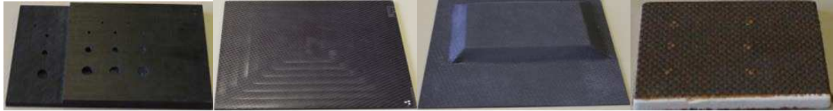
Figure 7: The four multi-layered and sandwich composite specimens
