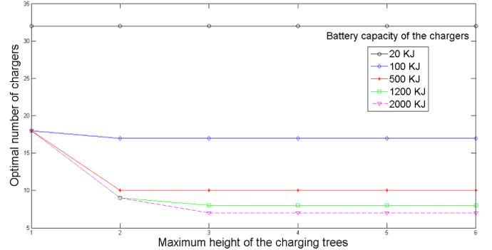
Fig. 2. The minimum number of chargers depending on the maximum height of the charging trees and the battery capacity of the chargers.
