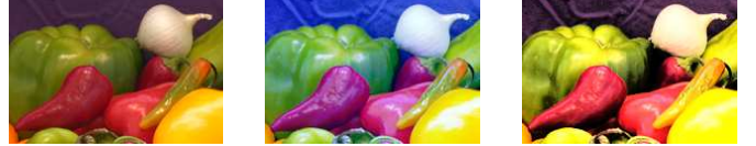
Fig. 1. Histogram equalization (HE). Left: Original image onion (Matlab IPT image credits notice). Middle: HE to each color channel independently. Right: Enhancement in three steps following [2]: RGB to HSI transform, HE of the intensity channel, then HSI to RGB transform. Here 36.1 % of the pixels have values in (255, 443.5].
