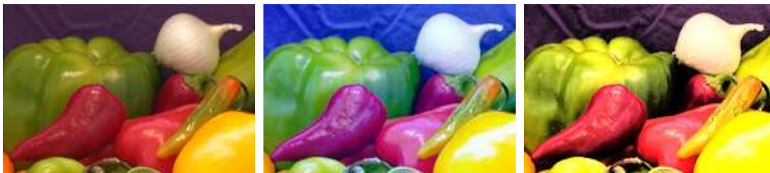
Fig. 1. Histogram equalization (HE). Left: Original image “onion.png” (Matlab IPT image credits notice). Middle: HE to each color channel independently – the colors are disturbed. Right: Enhancement in three steps following [4]: RGB to HSI transform, HE of the intensity channel, then HSI to RGB transform. Here 36.1 % of the pixels have values in (255, 443.5] ; they are clipped back on [0, 255] which yields too many yellow pixels.
