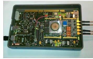
Figure 4. XtremeDSP Development board Kit-IV for Virtex-IV.
