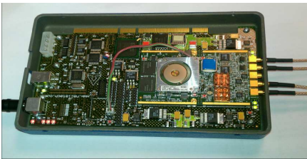
Figure 4. XtremeDSP Development board Kit-IV for Virtex-IV.
