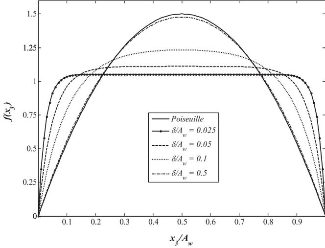
**Fig. 5.** Different types of profiles used to model the transverse variation of the velocity in our transversally confined cavity: Poiseuille profile (parabolic) and Hartmann-type profiles (13) for different values of  $\delta$ .
