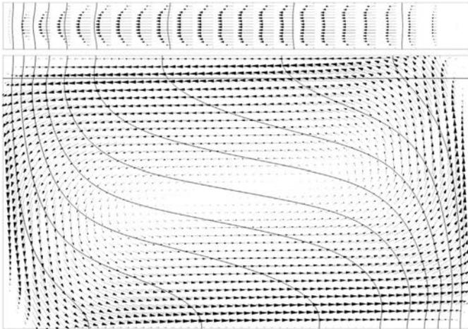
**Fig. 4.** Qualitative views of the velocity and temperature fields obtained from a 3D computation ( $Gr = 4.34 \times 10^6$  and  $Pr = 0.0129$ ) in the vertical middle plane (lower view) and in a horizontal plane (upper view). The vectors represent the velocity field. The lines are isotherms, except the horizontal straight line in the lower view, which gives the location of the horizontal cross section represented in the upper view.
