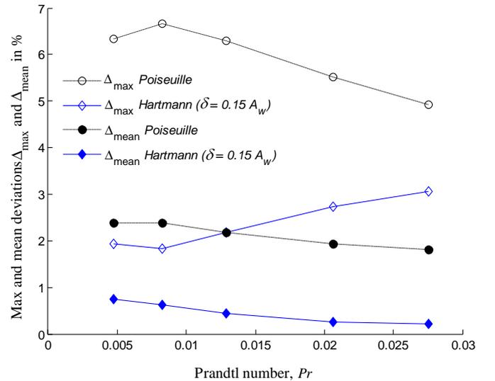
Fig. 9. Normalized maximum ( $\Delta_{max}$ ) and mean ( $\Delta_{mean}$ ) temperature deviations (in %) of the 2D½ simulations with respect to the 3D simulations as a function of the Prandtl number for  $Gr = 4.34 \times 10^6$ . Circles and diamonds correspond to 2D½ models featuring Poiseuille and Hartmann-type ( $\delta = 0.15 A_w$ ) profiles, respectively; solid symbols are for  $\Delta_{mean}$  and open symbols for  $\Delta_{max}$ .
