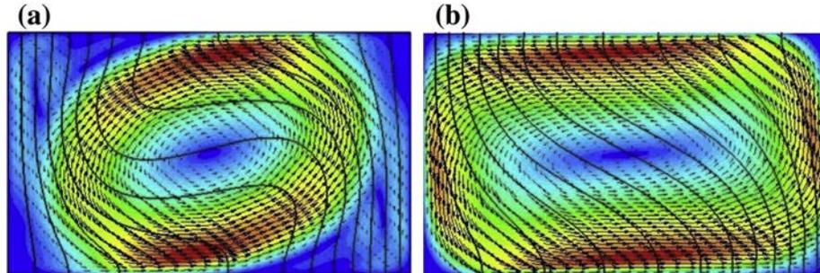
**Fig. 2.** Qualitative view of the velocity field (vectors and colours/grey levels) and temperature field (isolines) for  $Gr = 1.296 \times 10^6$  and  $Pr = 0.0129$ . On the left (2.a): snapshot of the 2D unsteady solution; on the right (2.b): 3D stationary solution in the vertical middle plane. (For interpretation of the references to colour in this figure legend, the reader is referred to the web version of this article.)
