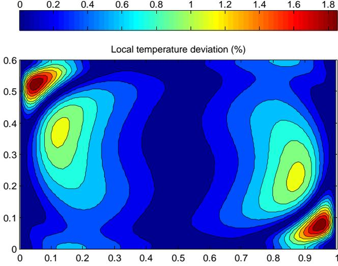
**Fig. 10.** Normalized deviation between the temperature field in the middle plane of a 3D simulation and the temperature field obtained from a 2D½-Hartmann simulation with  $\delta = 0.15 A_w$  for  $Gr = 4.34 \times 10^6$  and  $Pr = 0.0129$ .
