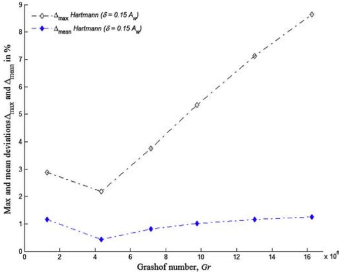
**Fig. 11.** Normalized maximum ( $\Delta_{\max}$ ) and mean ( $\Delta_{\text{mean}}$ ) temperature deviations (in %) of the 2D½-Hartmann model, with  $\delta = 0.15 A_w$ , with respect to the 3D simulations as a function of the Grashof number for  $Pr = 0.0129$ . Solid symbols are for  $\Delta_{\text{mean}}$  and open symbols for  $\Delta_{\max}$ .
