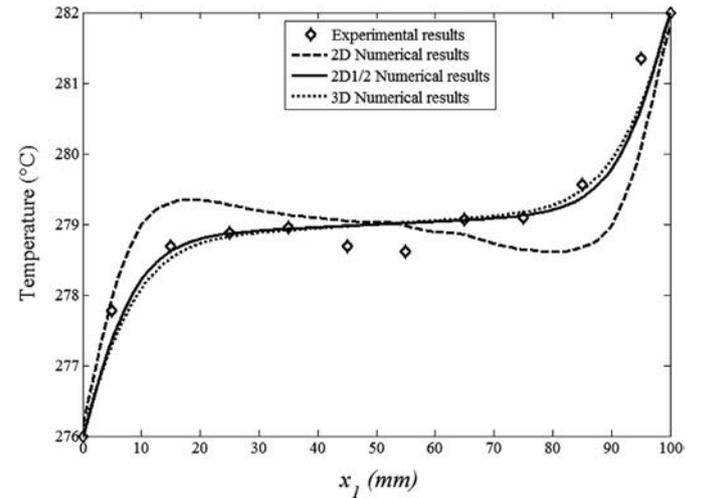
**Fig. 12.** Temperature profiles along  $\mathbf{x}_1$  at mid-height of the cavity ( $x_2 = 30$  mm) for the numerical and experimental results ( $Gr = 8.88 \times 10^6$  and  $Pr = 0.0152$ ). The Hartmann model with  $\delta/A_w = 0.15$  is used for the 2D½ simulations.
