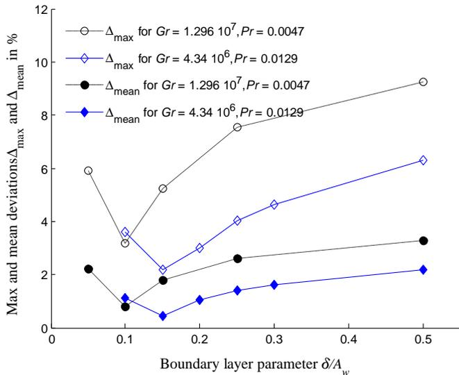
Fig. 8. Normalized maximum ( $\Delta_{max}$ ) and mean ( $\Delta_{mean}$ ) temperature deviations (in %) of the 2D½-Hartmann simulations with respect to the 3D simulation as a function of the boundary layer parameter  $\delta/A_w$ . The two reported cases correspond to  $Gr = 4.34 \times 10^6, Pr = 0.0129$  and  $Gr = 1.296 \times 10^7, Pr = 0.0047$ .
