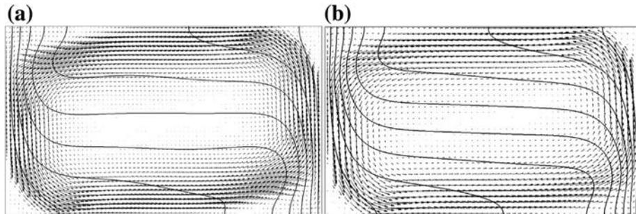
**Fig. 6.** Qualitative view of the velocity field (vectors) and isotherms for  $Gr = 1.296 \times 10^7$  and  $Pr = 0.0129$ . Left hand-side: 2D½ Poiseuille model (snapshot of the unsteady solution); right hand-side: 2D½ Hartmann model with  $\delta = 0.15 A_w$  (steady solution).
