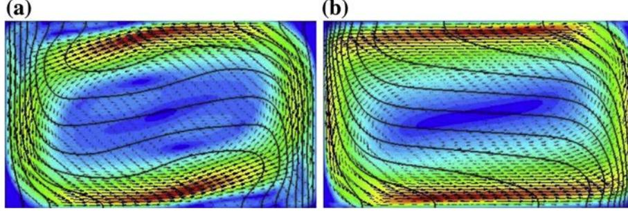
**Fig. 3.** Qualitative view of the velocity field (vectors and colours/grey levels) and temperature field (isolines) for  $Gr = 1.296 \times 10^7$  and  $Pr = 0.0129$ . On the left (3.a): snapshot of the 2D unsteady solution; on the right (3.b): 3D stationary solution in the vertical middle plane. (For interpretation of the references to colour in this figure legend, the reader is referred to the web version of this article.)
