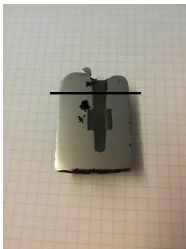
Figure 3. Cross section of the sample quenched 2 seconds after pure Mg addition; the reaction products were found above the black line.
