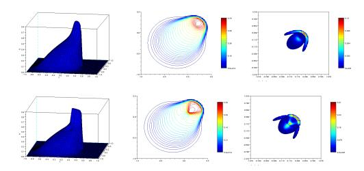
Fig. 4.13. Buckley-Leverett: 2D vs. Strang-split schemes, CFL=0.45 (top) & 0.95 (bottom).
