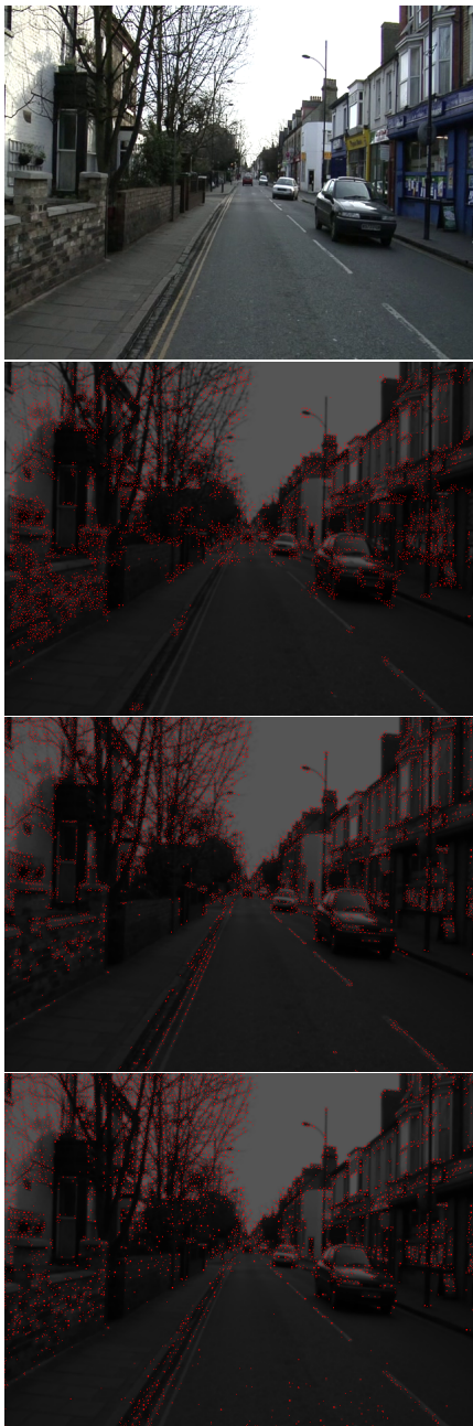
Fig. 3 From top to bottom: 1 - Test image of the detector benchmark. 2 - Points extracted with an ideal detector based on the matching error map (10k points with the smallest matching error). 3 - 10k FAST keypoints. 4 - 10k MIEL keypoints.
