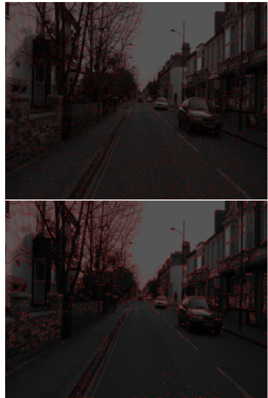
Fig. 2 Comparison of the local maximum (LM) selection (on the top) and the proposed strategy (on the bottom) using salience. In both cases, 9000 points are extracted using the MIEL salience (see Sec. 2.1.2). It turns out that, to get a high number of points, the LM method must select unreliable points, whereas our blockwise strategy provides a denser mapping of salient areas.
