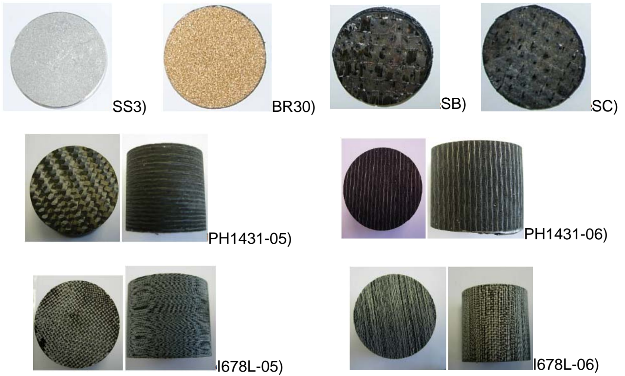
Figure 4. Pictures of porous media with corresponding denomination (SS: Stainless Steel and BR: Bronze with corresponding Poral class).
