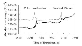
Figure 10. Energy by mass unit absorbed by the reactive fluid during the test with and without coke
