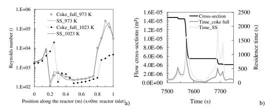
Figure 9. Hydraulic effect of coking formation (a) due to reduction of flow cross-section (b)
