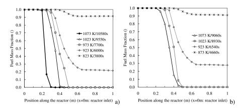
Figure 5. Computed dodecane pyrolysis profiles for each of the thermal plateaus: SS case (a) and Ti case (b)
