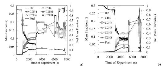
Figure 3. Computed chemical compositions of pyrolysis products: SS case (a) and Ti case (b).
