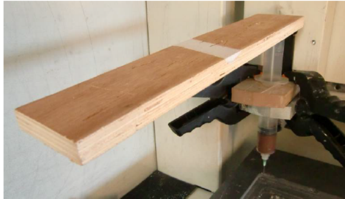
Figure 8 Syringe set on the computer numerical control (see online version for colours)
