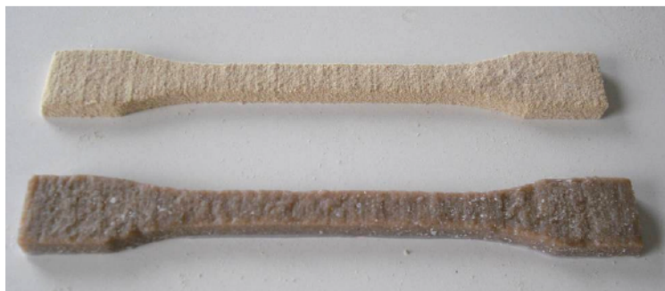
Figure 4 Specimen output printer (in fair) and post-treatment specimen (in dark) (see online version for colours)
