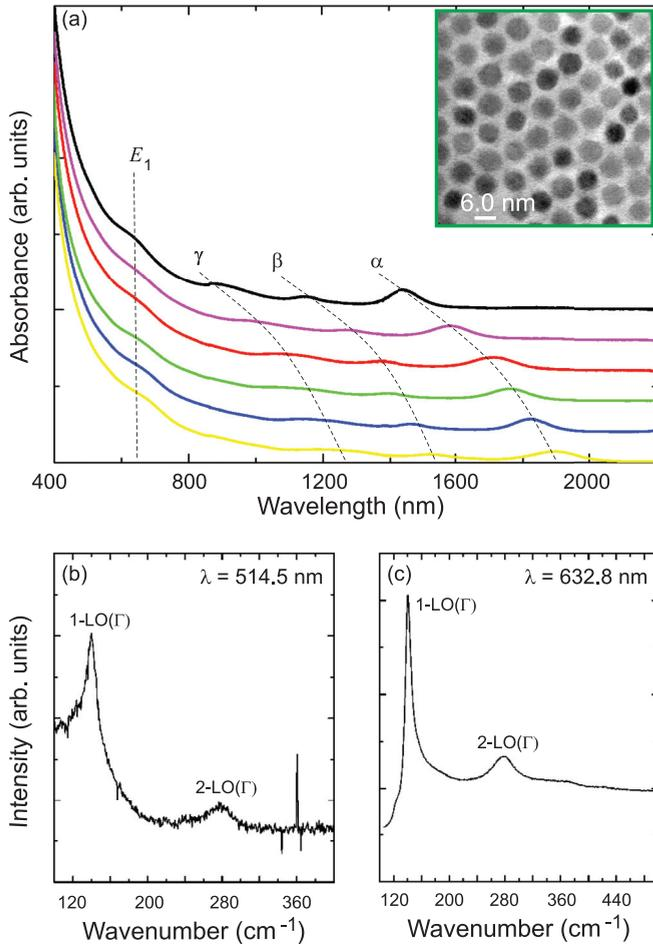
FIG. 1. (Color online) (a) Normalized absorbance spectra of PbSe nanocrystals for a range of mean diameter between 7.1 nm (bottom) and 4.5 nm (top). The optical transitions are labelled  $\alpha$ ,  $\beta$ ,  $\gamma$ , and  $E_1$ . Inset: TEM image of a monolayer of PbSe nanocrystals with a mean diameter of 6.0 nm. (b) and (c) Raman spectra of PbSe nanocrystals with a mean diameter of 6.8 nm for two optical excitation wavelengths.
