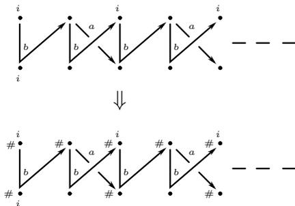
**Figure 4.6.** Computation of the vertices accessible from  $i$ .
