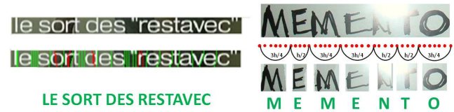
Fig. 14 Examples of recognized texts: the text on the left is recognized using the segmentation-based OCR and the text on the right is recognized using the segmentation-free OCR.
