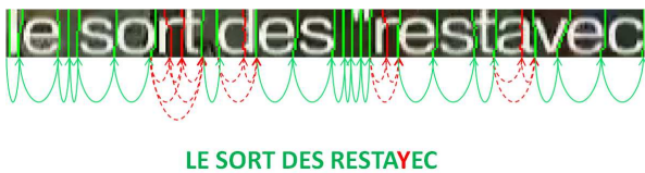
Fig. 6 An example of recognized texts: green arcs illustrate characters located between successive “accurate” segmentations and red arcs represent different possible configurations related to “risky segmentations”.
