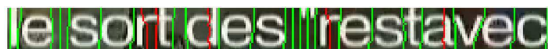
Fig. 4 An example of non-linear segmentations: “accurate” ones are shown in green and “risky” ones are shown in red.
