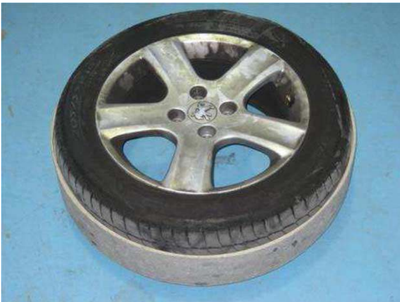
Figure 9. Skidconcept ring mounted on front wheel.
