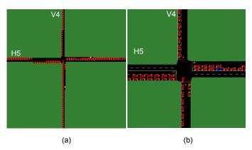
Fig. 14: A typical inefficient configuration in back-pressure control when capacities are not considered. The screen shot is captured at time 7135 with a population of 39000
