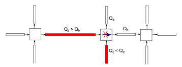
Fig. 5: Congestion propagation due to a loss of work conservation. Since  $N_b$  is full  $f_{ab}(k) = 0$  and  $N_a$  is not emptied, so congestion propagates to  $N_a$ . Moreover,  $N_c$  is also not emptied because vehicles do not have the right-of-way under the selected phase, so congestion propagates to both nodes  $N_a$  and  $N_c$ .
