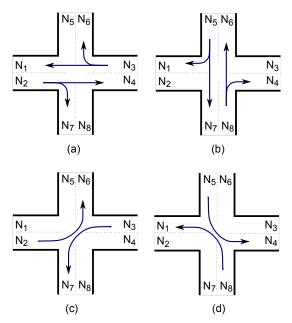
Fig. 2: A typical set of feasible phases at a junction. For phase (c), we have  $\mu_{26}(p^{(c)}) > 0$  and  $\mu_{37}(p^{(c)}) > 0$ .
