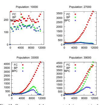
Fig. 13: Comparison of the average total time spent in the network through time under different population scenarios: 10000, 27000, 33000 and 39000. Time is in seconds. FC refers to the fixed-cycle control scheme, BP to back-pressure and BPC to capacity-aware back-pressure.
