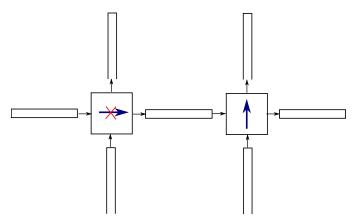
Fig. 3: Since the red-colored middle node is full, it cannot accept vehicles any more, even if the traffic light gives the right-of-way to vehicles going to this node.
