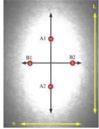
Figure 1. Screen shot of the diffraction image, indicating the position of the holes in the mask for signal detection by the quadrant detector (A1, A2, B1, B2) and the long (L) and short (S) axis of which the length is determined by the isointensity curves of the image analysis algorithm.
