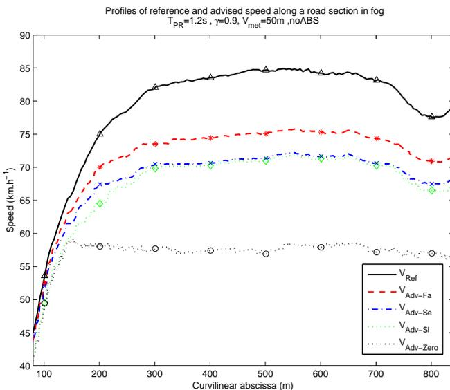
Fig. 12. Different speed profiles in fog with  $V_{Met} = 50$  m.
