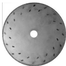
Fig. 1. A stone cutting disc with 2 \times 16 prestrained NiTi inserts designed by POMDI to alleviate stress concentrations in the rim during working conditions [6].
