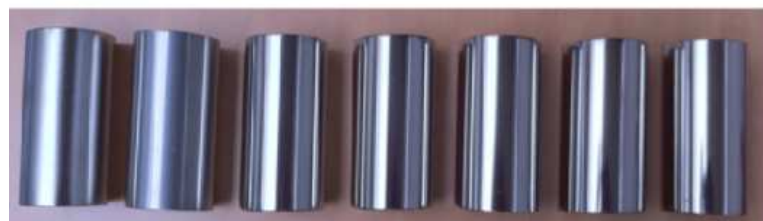
Figure 5 : Samples used for the evaluation of the accuracy of the Scanning From Heating
