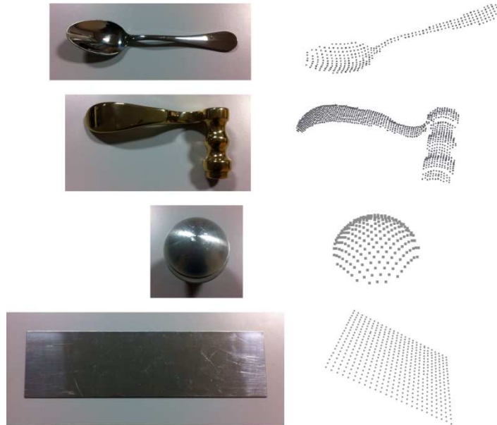
Figure 4 : Examples of 3D digitization results : polished steel, doorknob made of steel with a layer of brass, aluminum ball, steel plane
