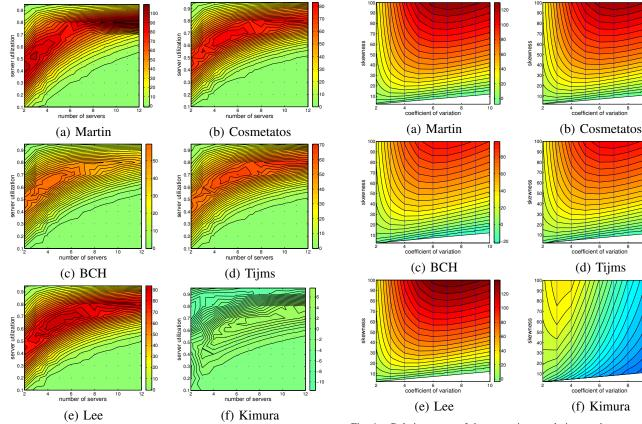
Fig. 3. Relative errors of the approximate solutions on the mean number of jobs in the M/Ph/m queue of example (B).
