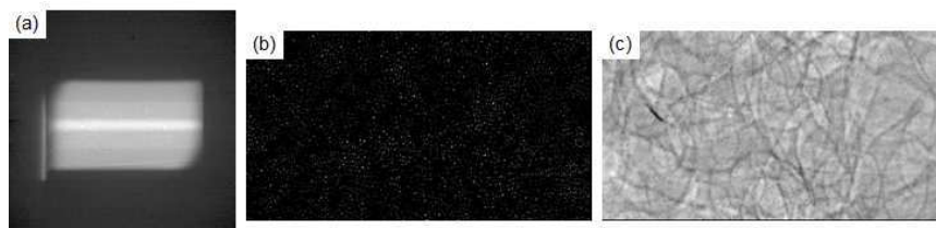
FIG. 6- (a) Initial image, (b) particle detection, (c) image of bubbles only
