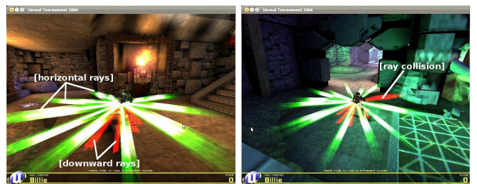
Fig. 4. Backup navigation based on ray casting
