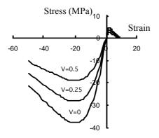
**Figure 2.** Constitutive law of a concrete as a function of the ageing variable V (stresses on the vertical axis are in MPa, strains on the horizontal axis are  $m/m \ 10^4$ )
