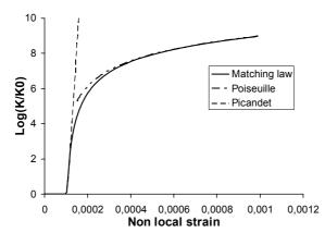
**Figure 6.** Logarithm of permeability evolution with state variable for the retained matching permeability law
