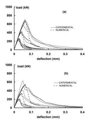
**Figure 3.** *Prediction of the response of leached beams for two leaching rates: a)* 45%; *and b)* 64%. *The thin lines correspond to the experimental results for each size and the thick lines correspond to the computations*
