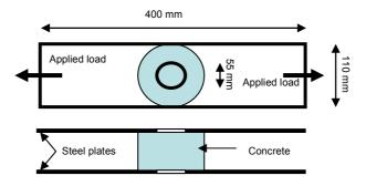
Figure 7. Bipede test geometry (after (Gérard, 1996))
