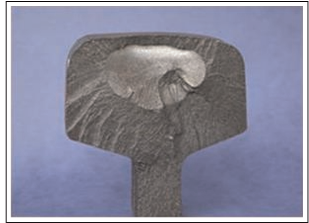
Figure 1. A broken rail owing to the spreading of an inner crack.
