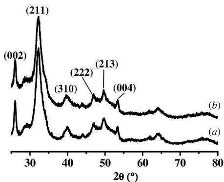
**Figure 2.** XRD diagrams for nanocrystalline apatite (NCA) powders before and after adsorption: (a) NCA and (b) NCA+BPs (equilibrium concentration at about 1.57 mM).
