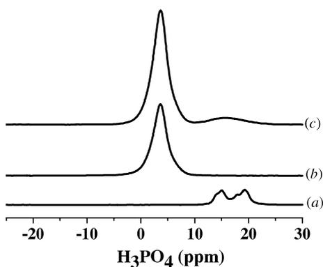
**Figure 6.**  $^{31}\text{P}$  MAS NMR solid-state spectra for tiludronate: (a) BPs and for NCA powders before and after adsorption: (b) NCA and (c) NCA+BPs (equilibrium concentration at about 1.57 mM).
