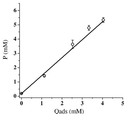
**Figure 8.** Concentration of phosphate ions in supernatants upon adsorption of tiludronate on NCA in 1 mM KCl solution at pH 7.4 and  $T = 37^\circ\text{C}$ .
