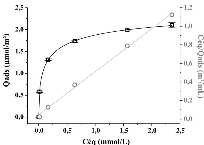
**Figure 7.** Adsorption isotherms of tiludronate by NCA from dilute aqueous solutions ( $\square$ ) and the corresponding linear regression of Langmuir ( $\circ$ ).
