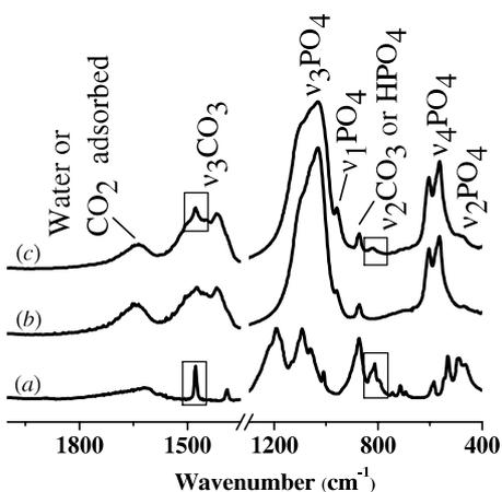
**Figure 3.** FTIR spectra for NCA powders before and after adsorption: (a) BPs, (b) NCA and (c) NCA+BPs (equilibrium concentration at about 1.57 mM).
