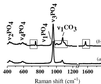
**Figure 5.** Raman spectra for NCA powders before and after adsorption: (a) NCA and (b) NCA+BPs (equilibrium concentration at about 1.57 mM).
